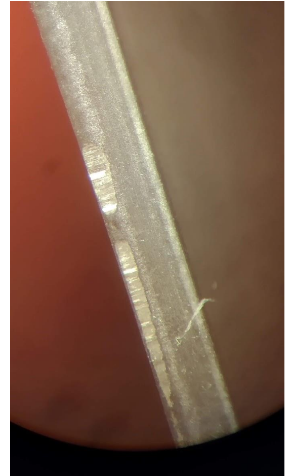
Fig. 9 Example of wear of a steel DLC coated vane
